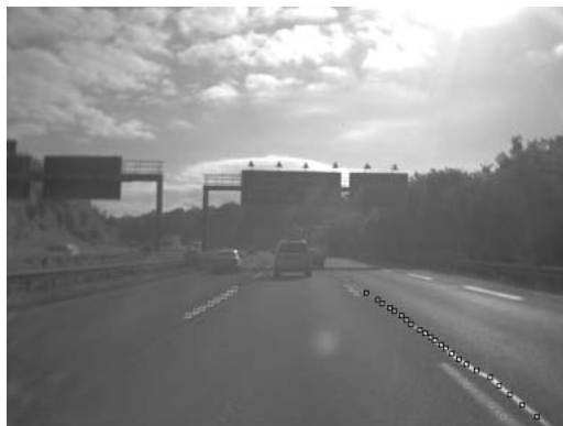
Figure 8.2: Lane detection by combining a specialized initial detection algorithm and an SCNN classifier. The initial detection produces points (indicated by small black boxes) which are conjectured to lie on a lane border. The classifier considers a small ROI around those points for its decision. Confirmed lane borders are indicated by bright boxes.
