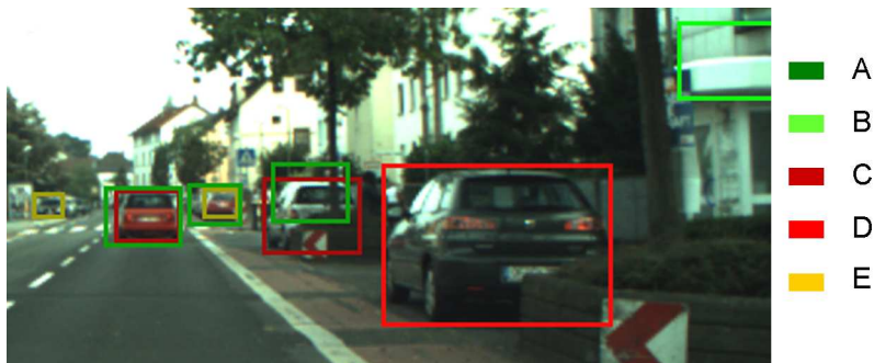
Figure 15: Example of single-image performance evaluation. A) Hypothesis matching an annotation (true positive case) B) hypothesis not matching any annotation in the current image (false positive case) C) annotation matched by one or more hypotheses D) annotation not matched by any hypothesis (false negative case) E) annotation that is not considered due to size constraints, see text. Such annotations do not constitute a false negative case when matched by a hypothesis, but neither a true positive case otherwise.
