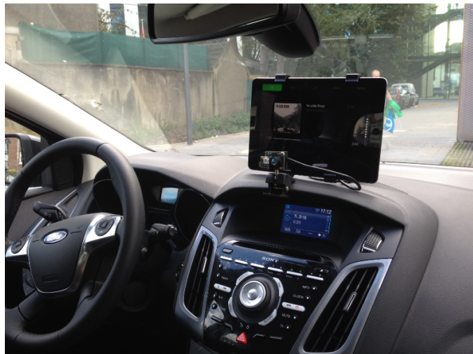
Fig. 7. Complete system: sensor, laptop and tablet mounted to the front console visualizing the infotainment system
